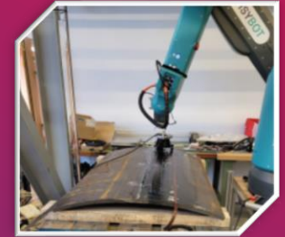
the cobot allows to move precisely and quickly the sensor on the surface of the part
