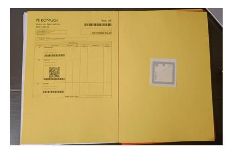
An NFC tag is implemented on the back of a Manufacturing Order.
