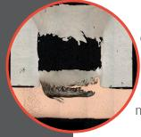
Creation of internal closed channels + joining to another component of same or different material in one single operation. Resulting in higher productivity and sustainable manufacturing solution.
